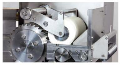
PRIMO 200 E with elastomer feed roll
